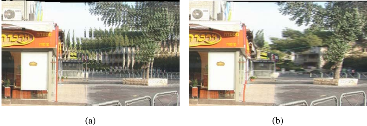
Figure 14: The benefit of stitching using dense depth. (a) A street view (X-slits) obtained by stitching without depth scaling. The restaurant (whose depth is close to the dominant depth in the scene) is stitched well, but closer and farther objects are truncated or duplicated. (b) Depth-based stitching eliminates duplications and truncations. Note that very narrow objects may still pose a problem for our method (Such as the narrow pole on the right side of the restaurant).
