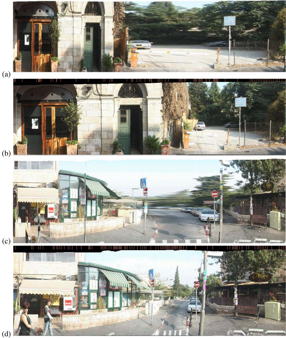
Figure 11: Pictures (a, c) are segments from a long pushbroom mosaic, while (b, d) show the same area in a long MAD mosaic. Substantial widening of far away objects and narrowing of close objects is evident in pushbroom. While width of strips is uniform in pushbroom, strip boundaries are marked on top of the MAD Mosaic image. Note also that the MAD mosaic avoids cutting inside moving objects.
