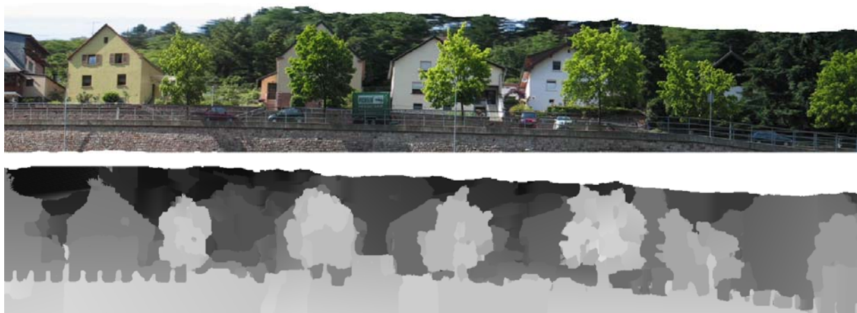
Figure 15: The panoramic image was constructed by X-Slits mosaicing from a sequence captured from a river boat. The corresponding panoramic inverse depth map is also shown.
